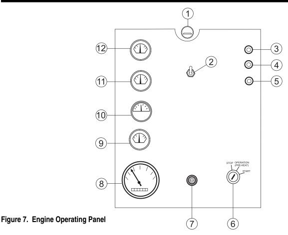
The definitions below describe the controls and functions of the DCA-45SSIU3 (60 Hz) "*Engine Operating Panel*" (Figure 7).
